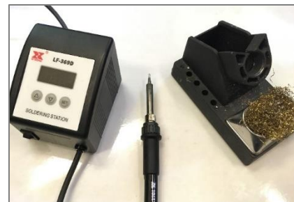
Figure 10: Temperature Controller Soldering Iron/station
