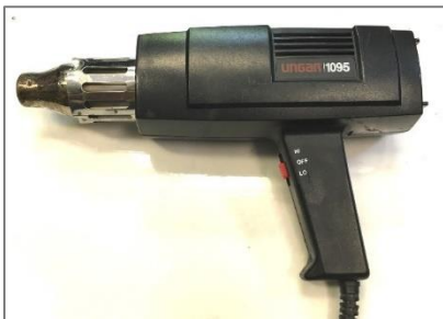
Figure 9: Heat Gun for Shrink wrap insulation
