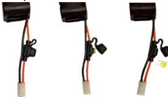
Figure 34: Fuse Removal
